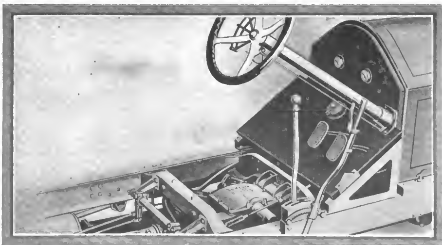
Fig. 2—Stoddard-Dayton chassis mid-section, showing control, clean dash and transmission
